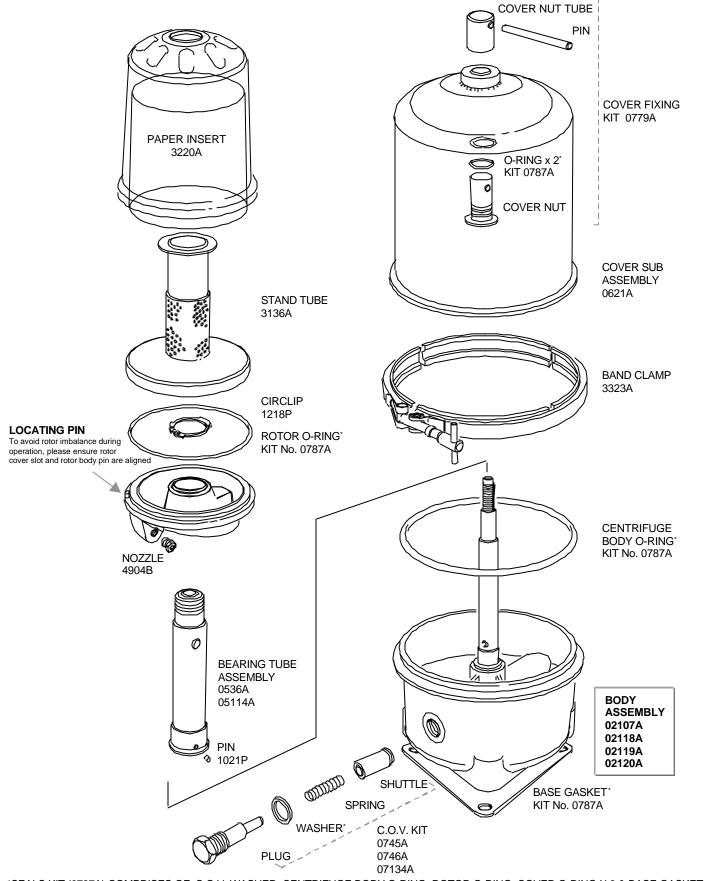
\*SEALS KIT (0787A) COMPRISES OF: C.O.V. WASHER, CENTRIFUGE BODY O-RING, ROTOR O-RING, COVER O-RING X 2 & BASE GASKET
